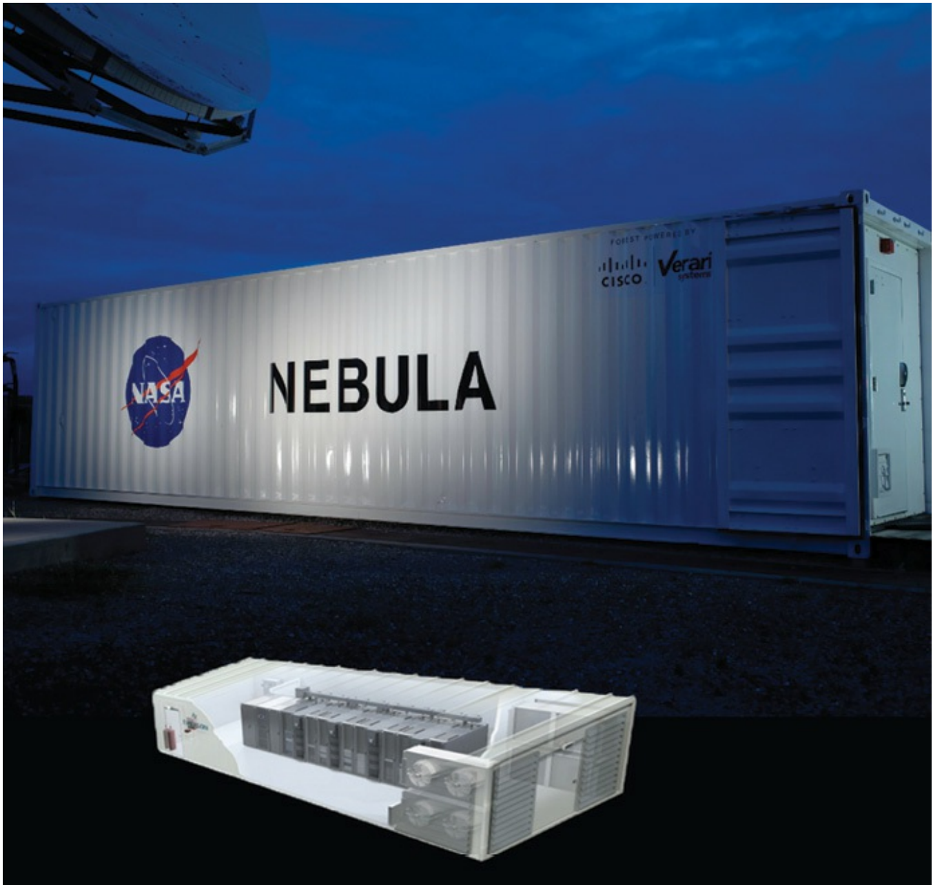
Figure 7.1 – An example of a Container Data Center module with a cutout of a typical interior layout. 24
