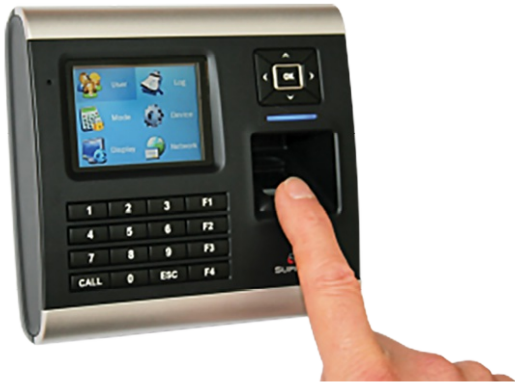
Figure 5.5 – A Fingerprint Reader scans the loops, whorls, and other characteristics of a fingerprint and compares it with stored templates. When a match is found, access is granted.
