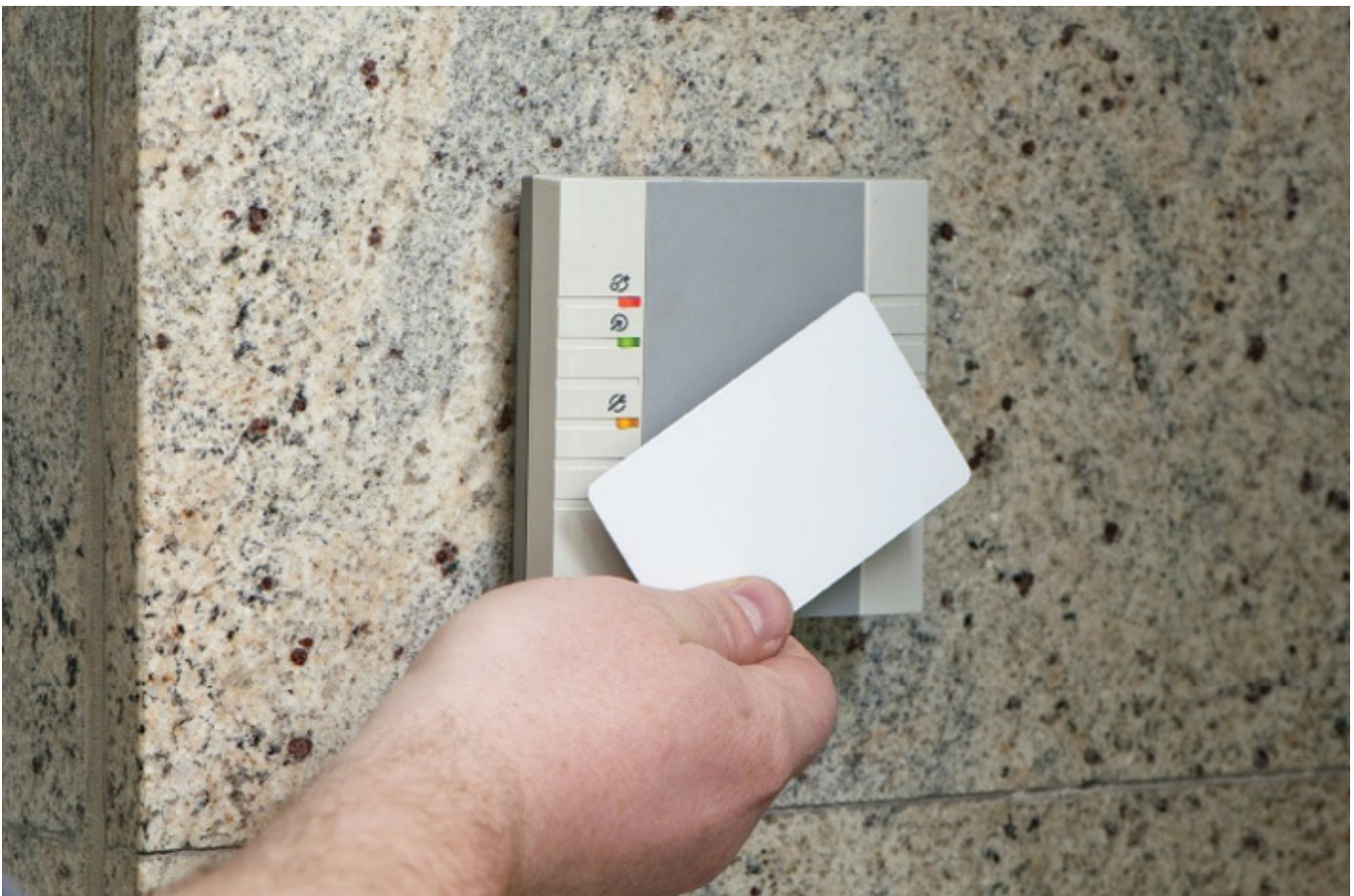
Figure 7.14 – A card reader is one of the basic components of an access control system.
