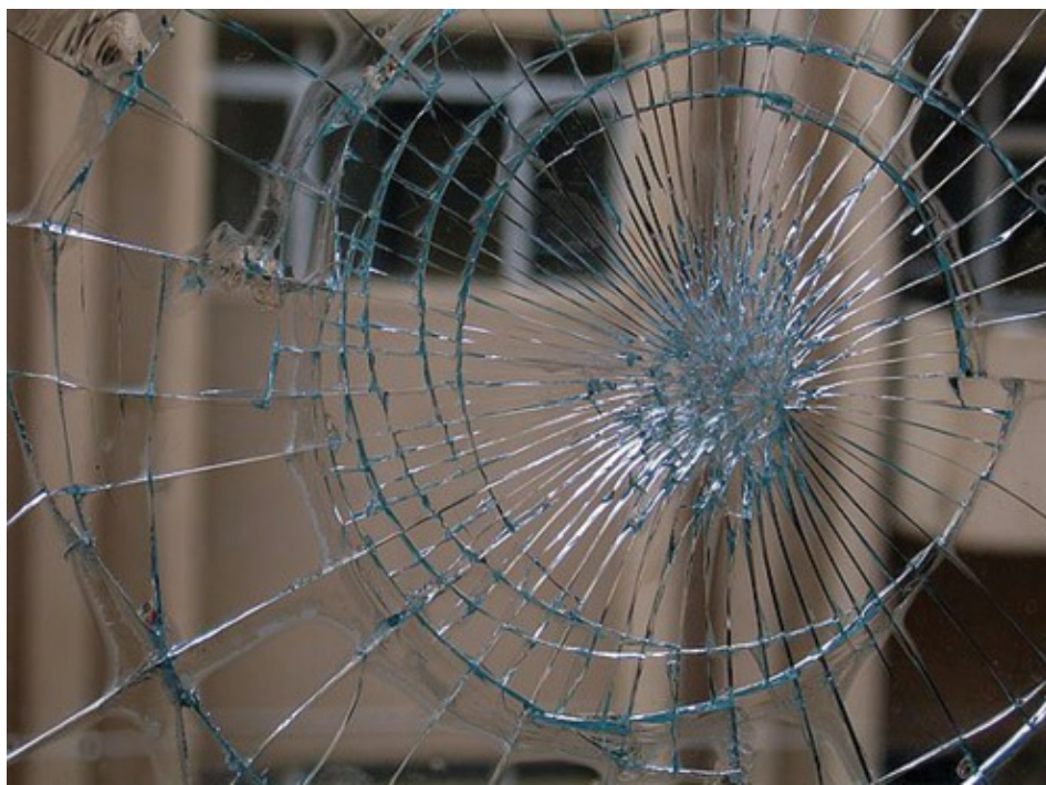
Figure 3.48 - Laminated glass is recommended for installation in street-level windows, doorways, and other access areas. (Courtesy of Bosch Security Systems)
